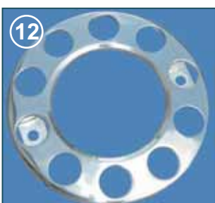
Stainless steel wheel nut cover ring 22,5" front new design - without visible rivets on the outside 12 10 hole rim, open 26mm bolt - for steel or aluminium rim with 26mm bolt hole for standard nuts Art. Nr. 2830917165016-26N 32mm bolts - for sleeve nuts Art. Nr. 2830917165016-32N
