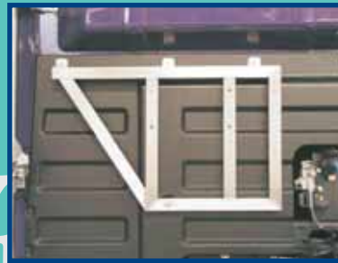
Mounting system for MB ACTROS MP 2 "Megaspacer" . Made of stainless steel to assemble on the driving cab rear wall (driver's side) without drilling to original fastening point! Art. Nr. 257V-11MB
