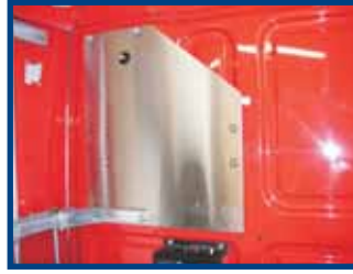
Mounting system for DAF XF made of stainless steel to assemble on the driving cab rear wall (driver's side) without drilling! Art. Nr. 257V-08DA
