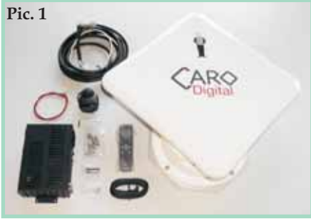
Pic. 1 - CARO Digital Mobile Satellite-System Complete Set for digital TV reception consists of : Digital-Receiver with integrated control logic. All TV + Radio programmes already stored. Turning plant with two specially-strong direct current motors for 24 +12 Volt. Independent lock by vehicle start. Height 13 cm - weight 14 kg. Mirror size Ø50cm. Art. Nr. 25209030015
