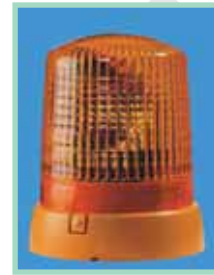
Flashing warning light KL7000F from Hella 24V, yellow, for fixed installation, H:194 Ø 155mm Rotation speed 160 T/min Noise suppression: capacityguide class 5 power input light bulb 70W Total power input 3,5A Art. Nr. 25609330034
