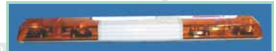
Flashing light bar Evolution Line -24V, 4 Module with free form reflectors, dual voltage, very high light output. Light hood made of shatter proof PC.- Labeling field opal, illuminable. Fastening with 4 stud bolts, incl.35mm rubber pad, complete wiring, incl. light bulbs 4xH. L 1524 x D 210 x H 108mm. Art.-Nr. 25609330032.3
