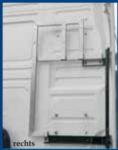
Mounting system for VOLVO Cab made of stainless steel to assemble on the driving cab rear wall (driver's side) without drilling and with original screws from cab. Art. Nr. 257V-10VO.right Art. Nr. 257V-10VO.left
