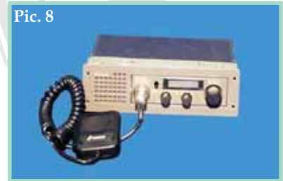
Pic. 6 - CB - radio equipment - Stabo xm 3003 3 changeable frequency tables: 80 FM (4W), 12 AM (1W) 40 FM (4W), 40 AM (1W) 40 FM (4W) CEPTsimply switch with border crossing. With module holder for DIN-Auto Radio-Stack Art. Nr. 25409010013.1 Without module holder Art. Nr. 25409010013
