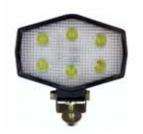
10-30 volt, 2600 lumens, 30 watt, 5 watt per LED, 6000K, IP67, 0,5 m cable
