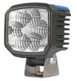
with 6 powerful LEDs, light output 850 lumens, 18 W, matt black aluminum housing with swivel base, without vibration damping, for standing or hanging mounting, protection IP6K7 and IP6K9K, ADR, 12/24V, W112 x H129 x D62 mm, Hella no. 1GA 996 188-001
