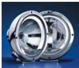
headlamp clear glass with integrated Celis® lighting technology (LED parking light ring), chrome housing, without bulb (H1), 12/24V, Hella no. 1F8 007 560-211
