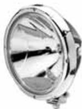
headlamp with position light (W5W), black plastic housing with design chrome frame, without bulb (H1), 12/24V, Hella no. 1F8 009 797-101
