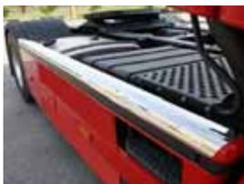
for the assembly on top of the side panel, 2 pieces for left & right side, for the assembly 3M tape and rivets are recommended (not included), stainless steel, highly polished
