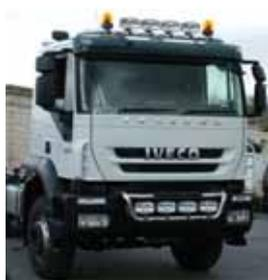
Stralis Active Time (low roof), with 5 white LEDs, pre wired for 4 headlamps and 2 warning lights, with holder for 4 headlamps, 63 mm pipe, in stainless steel or anodised aluminium
