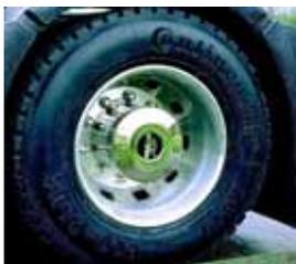
10 holes, pitch diameter 335 mm, for standard nuts and sleeve nuts. Vented high version, mounting at the wheel bolts, 218 mm from "axle bottom wheel to screws of axle cover", height of axle-cover: 240 mm, fits to MAN, Mercedes Benz, Iveco
