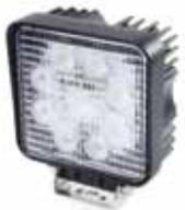
with 9 power LEDs 3 watt, 0,5 m cable, 10-30 volt, 1610 lumens, 27 watt, IP67
