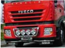
with 3 white LEDs, 63 mm pipe, with holder for 4 headlamps (e.g. Hella Rallye 3000), pre wired, with fitted orange side marker lights, with moulded rubber step, in stainless steel or anodised aluminium
