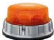
operating voltage 10-32V, power input max 30W, inverse-polarity protection, automatic brightness control, via switch selectable warning signal (rotating or flashing), no moving parts, extremely flat, ADR approved, Hella Nr. 2XD 011 557-101
