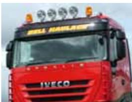
from model 2012 & Cube from model 2007 Active Space low roof, with 5 white LEDs, pre wired for 4 headlamps and 2 warning lights, with holder for 4 headlamps, 63 mm pipe, in stainless steel or anodised aluminium
