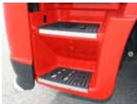
4 pieces for left & right side, stripes for the assembly at the steps with rivets (included), stainless steel highly polished
