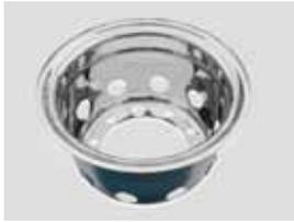
inch, universal (closed), for 1 wheel, without middle pan, screwed with original bolts. Measurement for rim's depth 285 mm, rim flange - rim base
