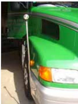
with sidelights or ballhead, with attractive bracket, lights are not allowed by the traffic code. The total width can be exceeded by the assembly
