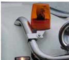
for assembly on the side of HiBars with drop down style (right)
