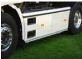
from model 2007, w/b tractor unit 4x2, with factory fitted sideskirts, wheelbase 3800 mm, with 5 amber LEDs on each side
