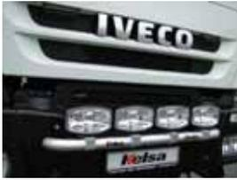
63 mm pipe, with holder for 4 headlamps, pre wired, with 3 white LEDs, in stainless steel or anodised aluminium
