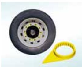
Checkpoint's are position indicators for loosened wheel nuts which are to mount at the nut itself. The indicators must stay face to face.
