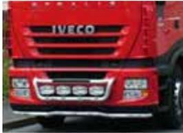
from model 2007, pre-wired with 5 white LEDs, doesn't fit for older Stralis models, in stainless steel or anodised aluminium
