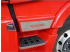
2 pieces for left & right side, assembly at the lower part of the doors, stainless steel highly polished
