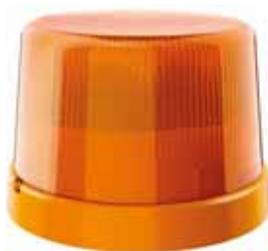
light cover & case in yellow, for fixed installation, speed 160 r/min, 10-32 V, X1-standard flash tube, ADR, total current 0.8 A, Hella no. 2RL 011 484-001
