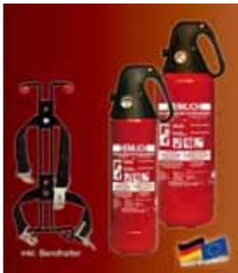
with support for cars - licensed DIN EN 3 for the fire classes A, B, C - performance 13A, 89B, and C - can be checked and refilled - spray length approx. 4 m., spray duration approx. 11 sec., dimensions with support H385 x B125 x T80 mm. GS-sign, CE-concurring (6 kg model not included)
