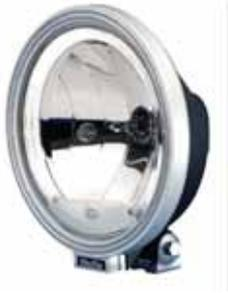
headlamp with integrated Celis® lighting technology (LED parking light ring), black plastic housing with silvergrey frame, without bulb, 12/24V, Ø224 mm, Hella no. 1F8 006 800-401
