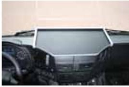
for 2300 mm width cab, fitted from model 2012, poplar plywood laminated, including anti-slip mat or coating
