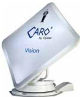
totally digital satellite system for digital TV reception, 50 x 50 x 13 cm flat antenna, Rotating system with 2 extra strong DC motors for 24 + 12 volt. Closes automatically when vehicle starts
