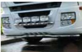
Active Time & Active Day, 63 mm pipe, with holder for 4 headlamps, pre wired, with 3 white LEDs, in stainless steel or anodised aluminium
