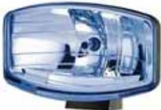
headlamp without positionlight, black plastic housing, clear glass, without bulb (H7), installation upright or hanging, 12/24V, W244,8 x H160,7 x D108,5 mm, Hella no. 1FE 008 773-061
